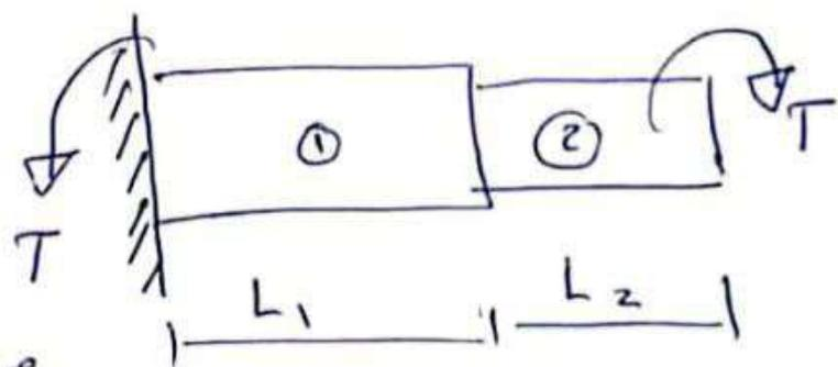
In such case each shaft transmits the same Torque and the total angle of twist is equal to the sum of the angle of twists of the two shaft
