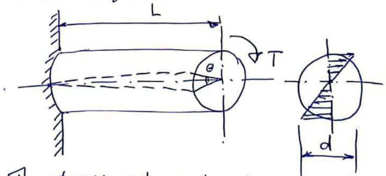
Note The stress set up by torsion is known as shear stress, It is zero at the centroidal axis and maximum at the outer surface.
