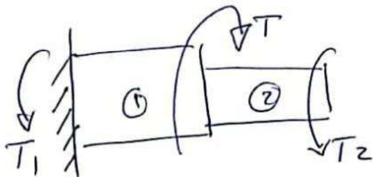
$$\frac{T_1 L_1}{C_1 J_1} = \frac{T_2 L_2}{C_2 J_2} \Rightarrow \frac{T_1}{T_2} = \frac{C_1}{C_2} \times \frac{J_1}{J_2} \times \frac{L_2}{L_1}$$
