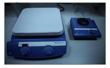
Magnetic stirrer is a device which provides mixing and keeping the chemical solutions and mixtures at a certain time and temperature by the help of a magneticbar.
