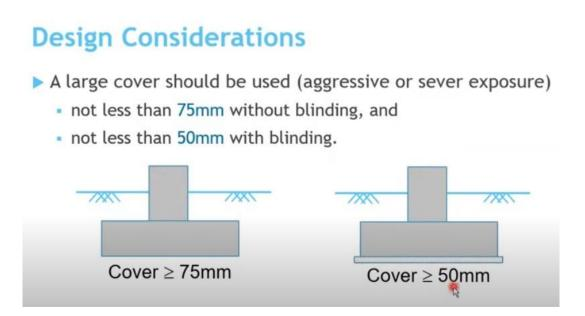
Use grade of concrete  $f_{cu} \ge 35 MPa$  =35000 KN/m2
