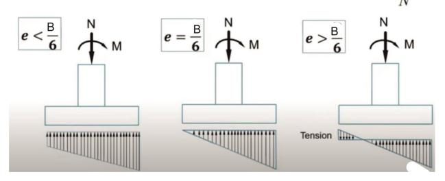
Never allow to use  $e > \frac{B}{6}$ , since the soil is weak in tension stresses.
