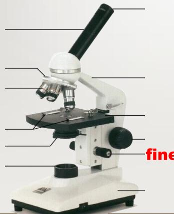
small, round knob on the side of the microscope used to fine-tune the focus of your specimen fine adjustment knob
