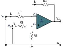
> If R1 = R2 = R3 = R4, then the circuit will become a **Unity Gain Differential Amplifier** and the transfer function for the differential amplifier will be
