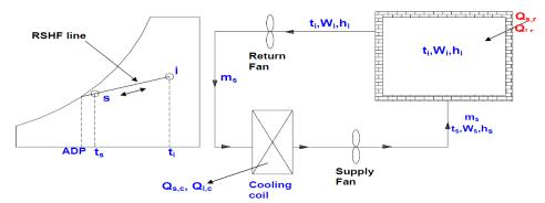
Fig.1: A summer air conditioning system with 100% re-cerculated air
