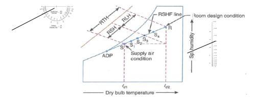
When the supply air conditions are not known, which in fact is generally required to be found out, the room sensible heat factor line may be drawn from the calculated value of room sensible heat factor (*RSHF*), as discussed below :
