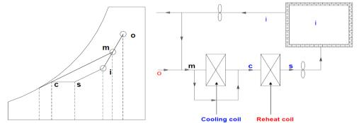
Fig.4: A summer air conditioning system with both reheat coil and by-pass factor for high latent cooling load applications
