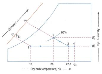
$v_{s1} = 0.81 \text{ m}^3/\text{kg}$  of dry air ... Mass of air supplied per minute,  $m_a = \frac{v_1}{v_{s1}} = \frac{15}{0.81} = 18.52 \text{ kg} / \text{min}$
