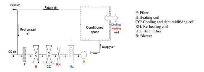
**Example 1:** An air conditioning plant is required to supply 60 m<sup>3</sup>/min at a DBT of 21 C and 55% RH. The outside air is at DBT of 28 C and 60%RH. Determine the mass of water drained and capacity of the cooling coil. Assume the air conditioning plant first to dehumidify and then to cool the air.
