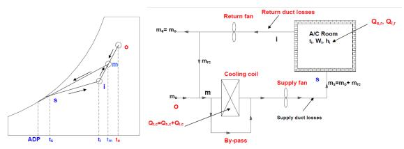
Fig.3: A summer air conditioning system with outdoor air for ventilation with by-pass factors
