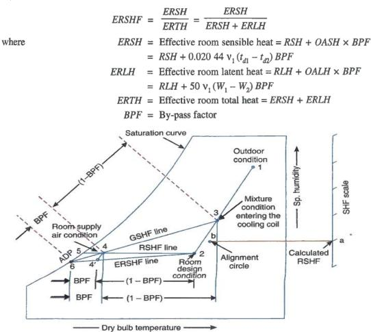
The line joining the point 2 and point 6 *i.e.* ADP, as shown in Fig. 18.17, gives the effective room sensible heat factor line (ERSHF line). From point 4, draw 4-4' parallel to 3-2. Therefore from similar triangles 6-4-4' and 6-3-2,
