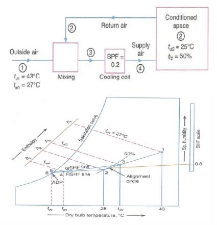
First of all, mark the outside condition of air at 43°C dry bulb temperature and 27°C wet bulb temperature on the psychrometric chart as point 1, as shown in Fig. 18.34. Now mark the inside conditions of air at 25°C dry bulb temperature and 50% relative humidity as point 2. We know that room sensible heat factor,
