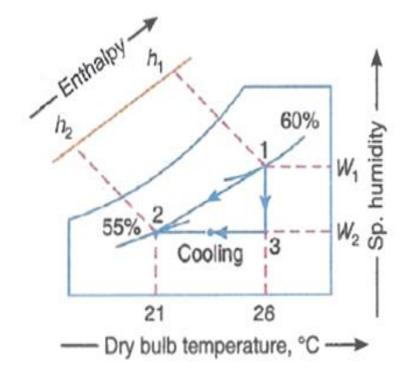
Mass of water drained =  $m_w = m_a(W_1 - W_2)$  $m_a = \frac{V}{v_{s2}}$ Capacity of cooling coil =  $C.C = m_a(h_1 - h_2)$
