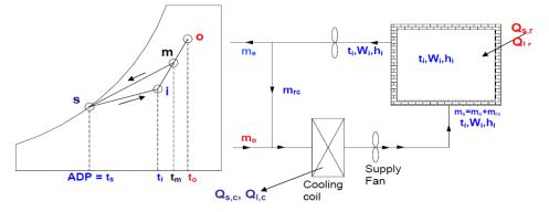
Fig.2: A summer air conditioning system with outdoor air for ventilation without by-pass factors
