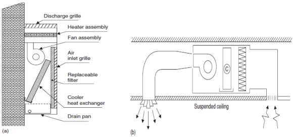
Figure: Fan coil units. (a)Wall mounted (b) ceiling mounted
