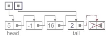
**3.** Dispose removed node.
