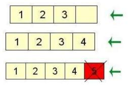
Fill it partially with some data. The array component without a number indicates allocated but unused space. This is space you could have used for something better. Add another element. We now have a full array to which we can not add any more elements. We can delete or replace, but we can not add.
