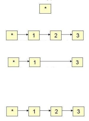
This is an empty linked list look like. The \* is an empty node (each element in a linked list called a **node**) which has its next-node reference set to the first node in the list. Since we don't have a first node, its next—node is a null pointer
