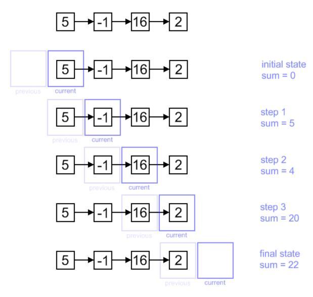
For some algorithms tracking the previous node is essential, but for some, like an example, it's unnecessary. We show a common case here and concrete algorithm can be adjusted to meet its individual requirements.
