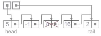
**1.** Update <u>next link</u> of the **previous node**, to point to the **next node**, relative to the removed node.
