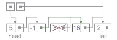
2. Dispose removed node.
