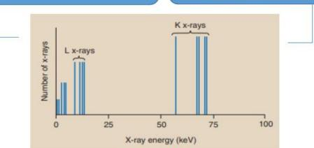
The maximum energy (in keV) of a Bremsstrahlung x-rays have a range of bremsstrahlung x-ray is numerically energies and form a continuous equal to the kVp of operation emission spectrum bremsstrahlung x-rays characteristic x-rays Number of x-rays Mo 19 25 69 75 50 100 0 X-ray energy (keV)
