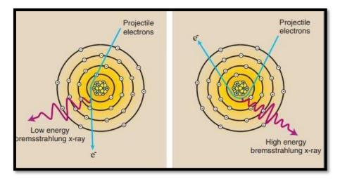
A projectile electron that completely avoids the orbital electrons as it passes through a target atom may come sufficiently close to the nucleus of the atom to come under the influence of its electric field (Figure below). Because the electron is negatively charged and the nucleus is positively charged, there is an electrostatic force of attraction between them
