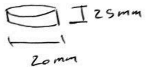
Ex-5 - In Fig. assume that a 20mm diameter rivet joins the plates that are each 110mm wide. The allowable stresses are 120 MPa for bearing in the plate material and 60 MPa for shearing of a rivet. Determine (a) the minimum thickness of each plate and (b) the largest average tensile stress in the plates.
