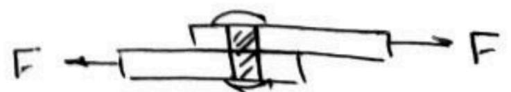
(b) largest tensile stress  $d = 20 \text{ mm}$
