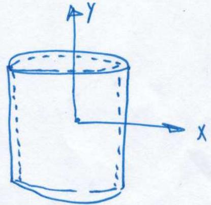
$$\sigma_y = \text{longitudinal stress} = \sigma_L$$
