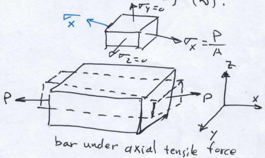
where  $\epsilon_x$  is strain in the x-direction and  $\epsilon_y$  and  $\epsilon_z$  are strains in the perpendicular direction, The (- sign) indicates a decrease in the transverse dimension when  $\epsilon_x$  is positive.
