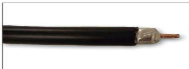
10BASE5 Thicknet Cable
