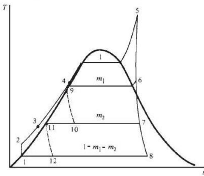
$$\diamond \text{ State 1 pump : } P_1 = 10 \text{ kPa} \quad \left. \begin{array}{l} h_1 = h_f @ P_1 = 191.81 \text{ kJ/kg} \\ v_I = v_f @ P_1 = 0.00101 \text{ m}^3/\text{kg} \\ s_I = 0.6492 \text{ kJ/kg K} \end{array} \right\}$$
