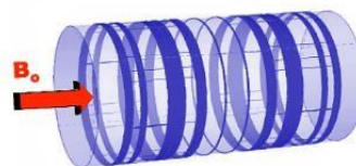
Rather than a single large/continuous winding, 6-10 large and small solenoidal bands are typically placed to create a more uniform central field with minimized fringe.
