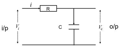
$$V_{\rm c} = \frac{1}{\text{RcD} + 1} V_i$$
