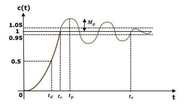
All the time domain specifications are represented in this figure. The response up to the settling time is known as transient response and the response after the settling time is known as steady state response.
