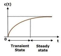
Here, both the transient and the steady states are indicated in the figure. The responses corresponding to these states are known as transient and steady state responses.
