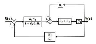
Step 3 – Use Rule 1 for blocks  $(G_3+G_4)$  and  $G_5$ . The modified block diagram is shown in the following figure.
