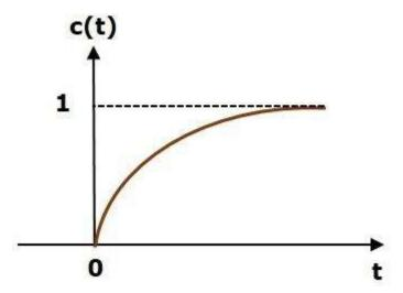
The value of the **unit step response**, c(t) is zero at t = 0 and for all negative values of t. It is gradually increasing from zero value and finally reaches to one in steady state. So, the steady state value depends on the magnitude of the input.
