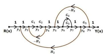
With the help of Mason's gain formula (discussed in the next chapter), you can calculate the transfer function of this signal flow graph. This is the advantage of signal flow graphs. Here, we no need to simplify (reduce) the signal flow graphs for calculating the transfer function.
