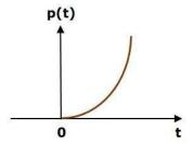
So, the unit parabolic signal exists for all the positive values of 't' including zero. And its value increases non-linearly with respect to 't' during this interval. The value of the unit parabolic signal is zero for all the negative values of 't'.
