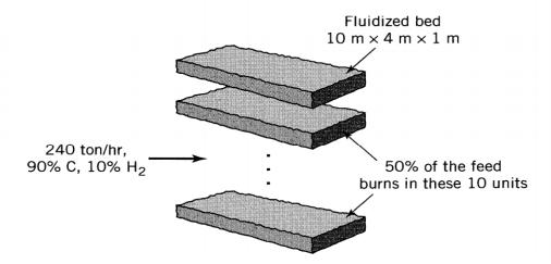
H<sub>2</sub>), 50% of which would burn within the battery of primary fluidized beds, the other 50% elsewhere in the system. One suggested design would use a battery of 10 fluidized beds, each 20 m long, 4 m wide, and containing solids to a depth of 1 m. Find the rate of reaction within the beds, based on the oxygen used.
