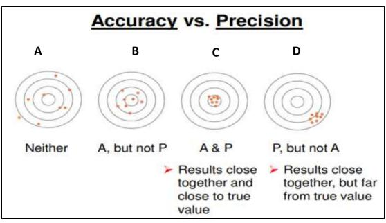
The picture showed the difference between accuracy and precision using the target-shooting metaphor. (A) is neither accurate nor precise because the shots are not close to the bull's-eye but all over the place. (B) is precise because the shots are clustered together, but not accurate because they are not close to the target. (C) is both accurate and precise, (D) is precise because the result close together but not accurate because far from the target .
