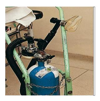
Entonox is compressed into cylinders to a pressure of 13 700 kPa. Entonox cylinders should be stored at 10°C for 24 hours before use. If the temperature of the Entonox cylinder is decreased to below°5.5- C, liquefaction and separation of the two components occur (Poynting effect). **This results in:**
