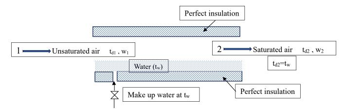
Adiabatic process in which no external heat flows in or out of the system, but interchange of energy can occur. Water is supplied at  $(t_w)$ . If the chamber is long enough and the water surface is adequate, experiments show that air leaves in a saturated state and at dry bulb temperature equaling the initial wet bulb temperature. i.e.  $t_{w1}=t_{w2}$ .
