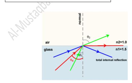
Optical fibers are based on this principle of total internal reflection. An optical fiber is a flexible strand of glass. The light travels along the optical fiber, reflecting off the walls of the fiber. With a straight or smoothly bending fiber, the light will hit the wall at an angle higher than the critical angle and will all be reflected back into the fiber.
