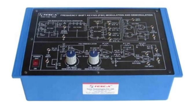
**Object:** To study the generation of the frequency shift keyed output and also to demodulate the FSK output.
