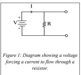
circuit element (like a light bulb) can act as a resistor. For experiments and for building circuits, small resistors of known resistance can be added to the circuit.
