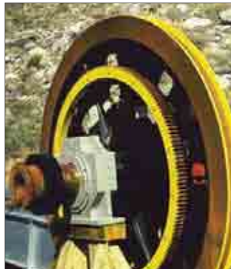
Wheel that winds the metal rope.
