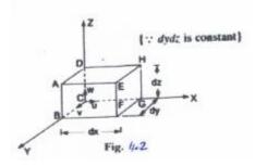
Mass of fluid entering the face ABCD=  $\rho V_x A = \rho u (dy \times dz)$ Mass of fluid leaving the face EFGH =  $\rho u dy dz + \frac{\partial}{\partial x} (\rho u dy dz) dx$ Gain of mass in x – direction = Mass through ABCD – Mass through EFGH
