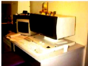
The image processing system of a gamma camera.
