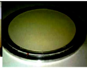
The NaI crystal of a gamma camera.
