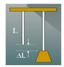
❖ An elastic deformation (strain) is directly proportional to the magnitude of the applied force per unit area (stress).
