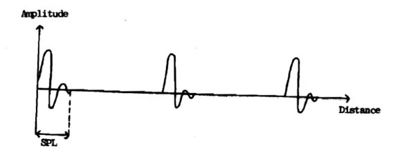
The wavelength remains constant, but the amplitude decays with distance. The oscillations eventually cease altogether after a distance known as the spatial pulse length (SPL). The SPL is the product of wavelength and the number of wave cycles constituting the pulse.
