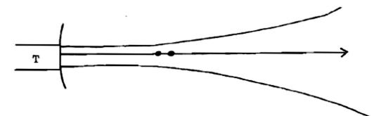
It is sometimes referred to as depth resolution. Lateral resolution is the ability to distinguish between two reflectors situated side by side in a direction perpendicular to that of the ultrasound beam.
