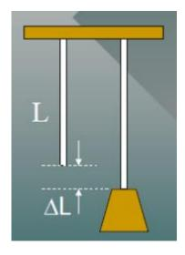
❖ An elastic deformation (strain) is directly proportional to the magnitude of the applied force per unit area (stress).
