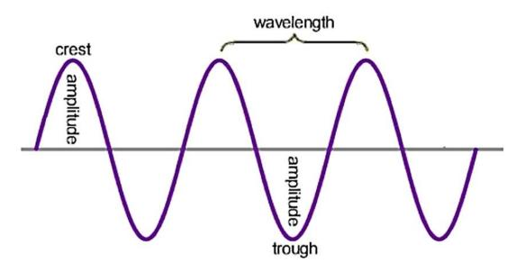
Wavelength is a measure of the distance from the crest on one wave to the crest on the very next wave.
