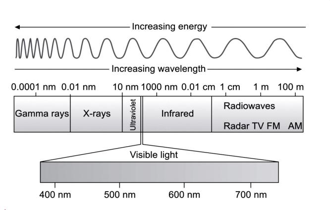
All of them travel at a velocity 'c' in a vacuum. The wavelength and photon energy of the whole range of electromagnetic radiation are summarized in Table.
