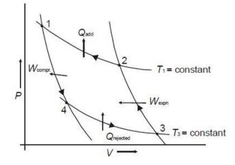
Heat engine cycle in reversed form as shown above is used as an ideal cycle for refrigeration and called "Carnot refrigeration cycle".
