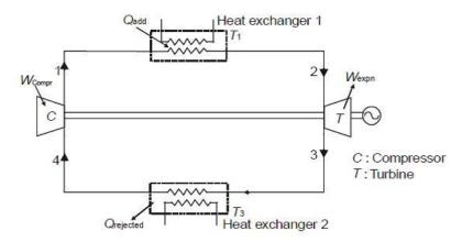
Carnot cycle can also operate reversibly as all processes constituting it are of reversible type. Reversed Carnot cycle is shown below.
