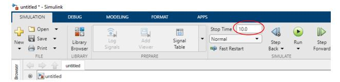
The default stop time of 10.0 is appropriate for this model. This time value has no unit. The time unit in Simulink depends on how the equations are constructed.
