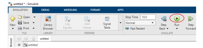
The simulation runs and produces the output in the scope viewer.
