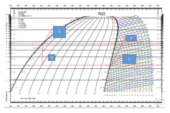
We extend a line from each point to the chart where the enthalpy readings are
