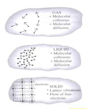
4 The basic equation for thermal conduction is the **Fourier's law**.
