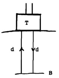
> To determine the distance d of the reflector, we use the simple relationship.
