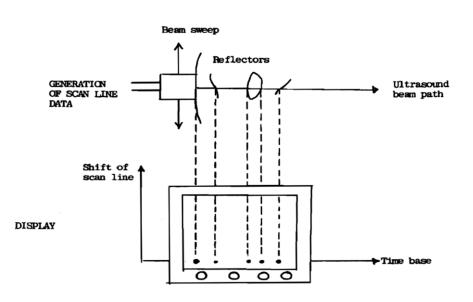
Fig illustrates the relationship between the positions of scan lines and the display of dots on the CRO to build the 2-D image.
