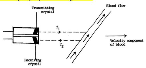
The distance of a moving structure from the transducer cannot be determined by CW ultrasound, since the go-return time for the ultrasound beam will not be known. Determination of range requires the use of pulsed beams. More sophisticated Doppler shift equipment utilizes PW ultrasound in conjunction with B-mode scanning to detect movement and determine range, and to produce images of regions of movement.
