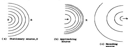
The apparent difference in frequency is called the Doppler shift. For a stationary source, the wave fronts are neither compressed nor stretched, hence no shift of frequency is observed. The Doppler shift can be measured and used to:
