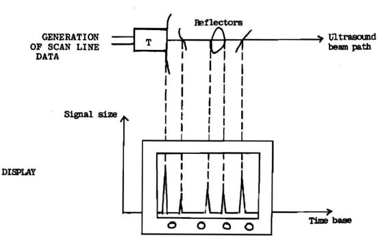
On one axis (vertical axis) the amplitude of the signal (magnitude of the voltage pulse) is displayed, and on the other axis (horizontal), the position of the signal on a time scale is represented.
