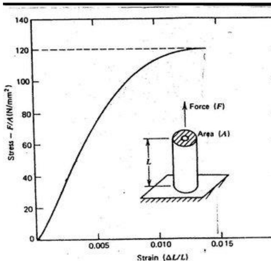
Scheme [1] When A Piece of Bone Placed under Increasing Tension, Its Strain  $\Delta L/L$  Increases Linearly at First (Hooks Law) And Then More Rapidly Just before It Breaks in two at  $120 \text{ N/mm}^2$
