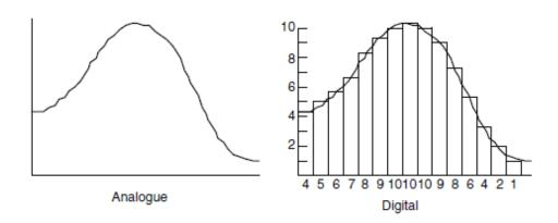
• The input to the ADC is an analogue signal whose amplitude varies continuously with time, and the output is a corresponding stream of binary numbers as illustrated in figure below.
