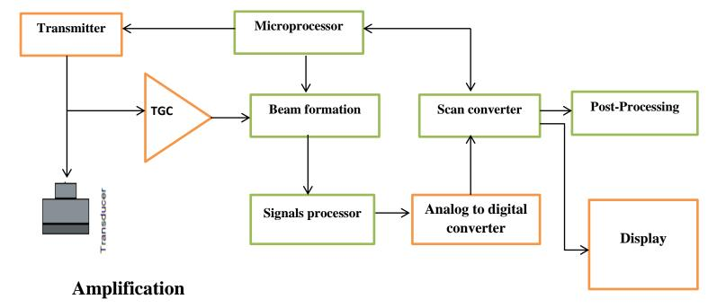
The echo signals generated at the transducer elements are generally too small in amplitude to be manipulated and displayed directly and need to be amplified (made bigger).
