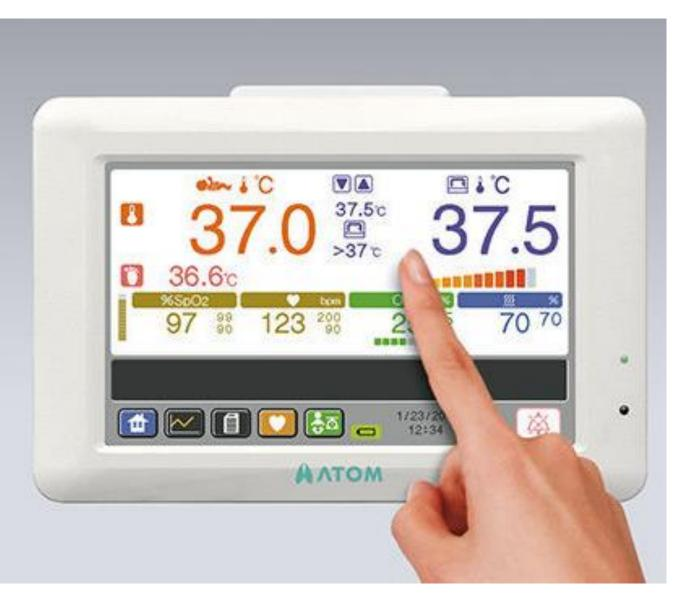
•In order maintain the body temperature of the baby (30 - 37.2°C) the incubator must be able to create an ambient air of 34 - 38°C with a humidity of 40 - 80%.
