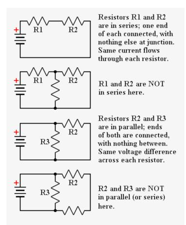
Figure 3. Series and parallel connections.
