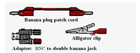
Figure 3. Typical connectors used in an introductory physics laboratory.
