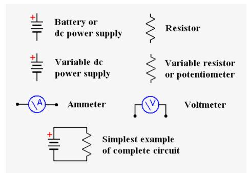
Figure 1. Schematic symbols for simple circuit elements.
