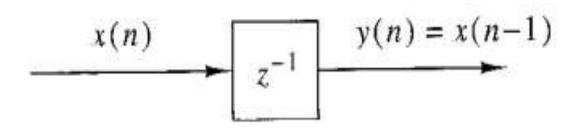
Graphical representation of the unit delay element
