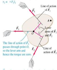
$\vec{F}_2$  tends to cause *clockwise* rotation about point O, so its torque is *negative*:  $\tau_2 = -F_2 l_2$
