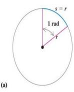
An angle  $\theta$  in radians is the ratio of the arc length s to the radius r.
