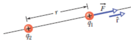
Figure 3: The electrostatic force on particle 1 can be described in terms of a unit vector along an axis through the two particles, radially away from particle 2.
