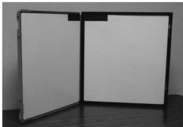
Figure (4) Typical set of intensifying screens inside a cassette.
