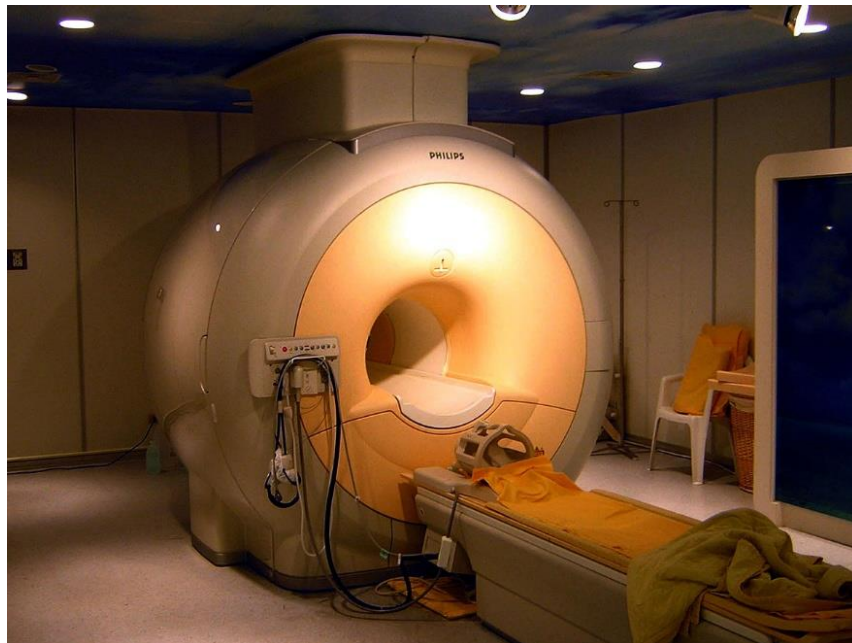
Fig. 1 Clinical MRI system with the patient table in the front that can be moved inside the bore of the magnet.
