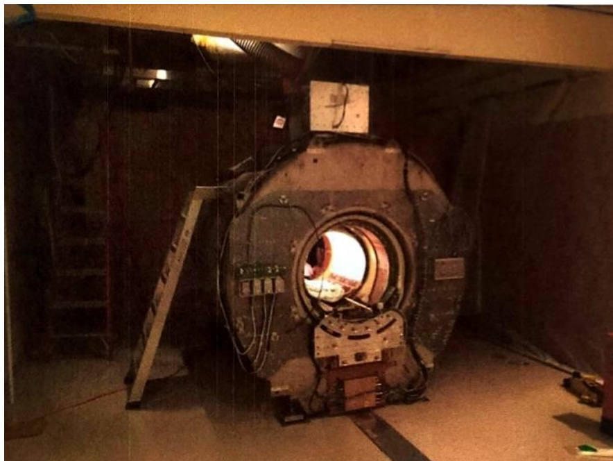
Fig. 2 Superconducting magnet of a clinical MRI system after the removal of the covers and the patient table.
