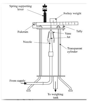
Fig 11.1 Impact of Jet Apparatus
