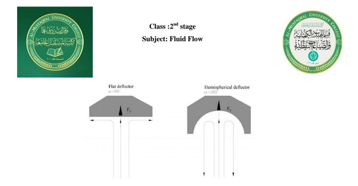
Fig 11.2 Examples of flow deflection angles for flat and hemispherical deflectors From equilibrium of forces in a vertical direction,  $F_y$  is balanced by the applied weight on the weight pan, W (W = mg, where m is the applied mass), i.e.,  $F_y = W$ . Therefore:
