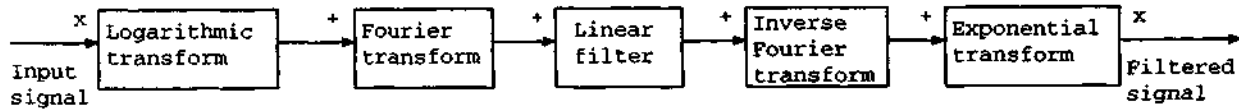
Figure 4.20 Operations involved in a multiplicative homomorphic system or filter. The symbol at the input or output of each block indicates the operation that combines the signal components at the corresponding step.
