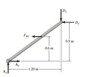
**Example No. 3:** The frame shown in Figure is supported by a hinge at A and a roller at E. Compute the horizontal and vertical components of the hinge forces at B and C as they act upon member ABC.
