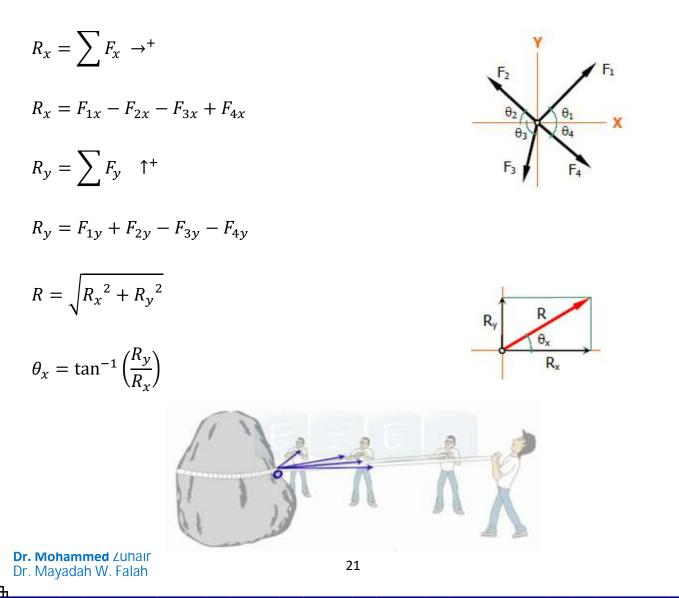
**Example No. 1:** Determine the magnitude and direction of the resultant forces system shown in Figure.
