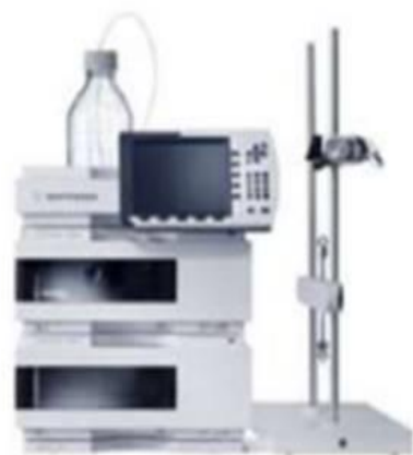
Modular HPLC System – basic configuration with isocratic pump, manual injector, variable wavelength detector, and hand-held controller
