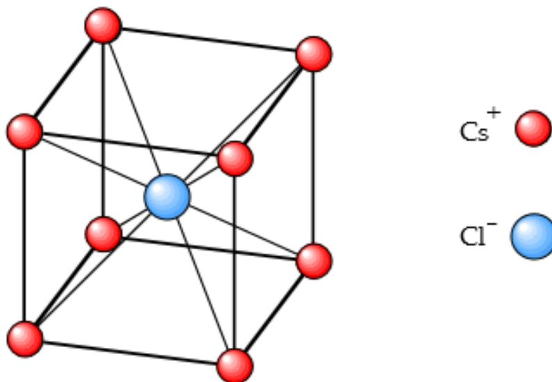
■ Cesium chloride crystallizes in a cubic lattice. The unit cell may be depicted as shown. (Cs<sup>+</sup> is teal, Cl<sup>-</sup> is gold)
