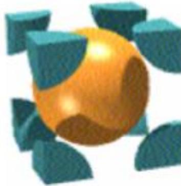
■ Cesium chloride consists of equal numbers of cesium and chlorine ions, placed at the points of a body-centered cubic lattice so that each ion has eight of the other kind as its nearest neighbors.
