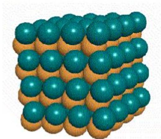
The translational symmetry of this structure is that of the simple cubic Bravais lattice, and is described as a simple cubic lattice with a basis consisting of a cesium ion at the origin 0 and a chlorine ion at the cube center
